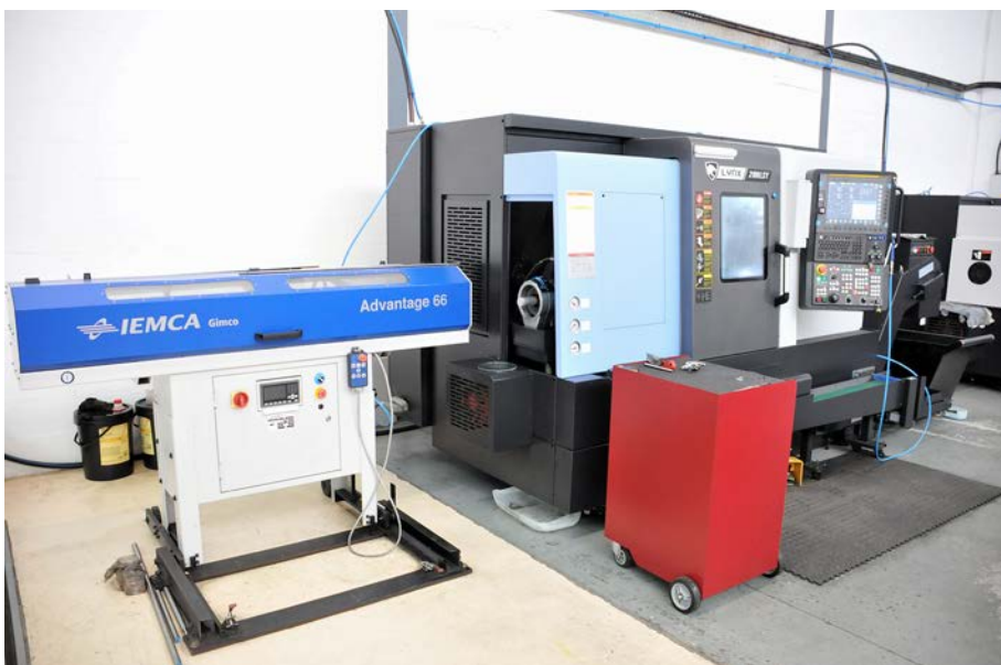
The company also has a Lynx 2100LSYB, which is a high-performance mill-drill turning center that combines Y-axis milling, live tooling, a synchronised sub-spindle, and full C-axis contouring and a Puma DNT 2100M CNC lathe with XY travels of 230mm by 580mm, maximum swing diameter of 650mm, maximum turning diameter of 320mm and a maximum turning length of 513mm. The Lynx has an lemca Advantage 66 bar feeder attached to it. All of these machines were supplied by Puma Machine Tools
