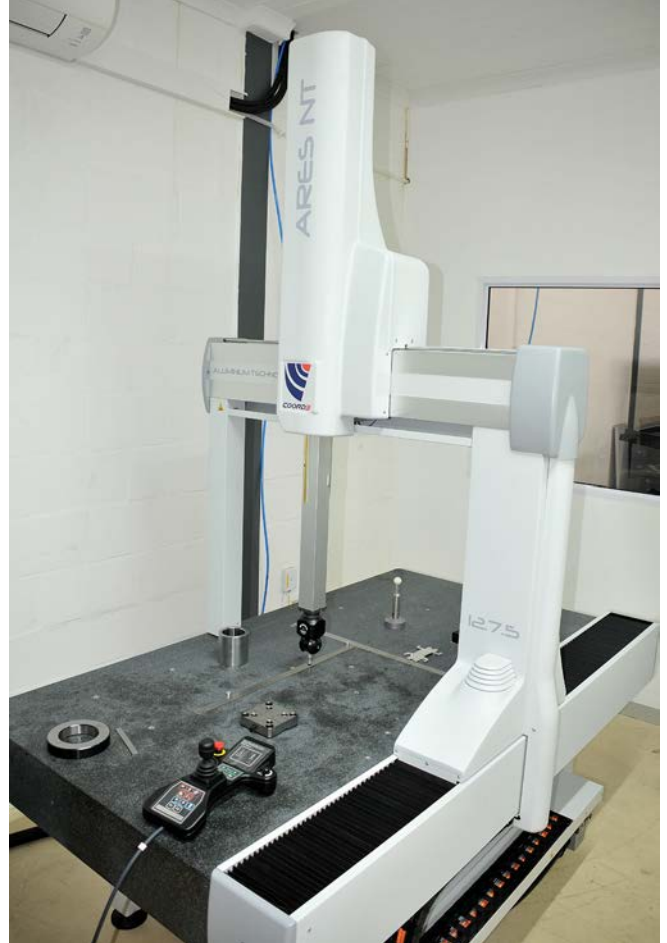
Another recent purchase is the COORD3 ARES NT, which is a high-precision, small-to-mid-sized bridge-type CMM
