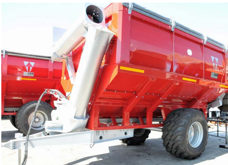
A chaser bin being assembled
