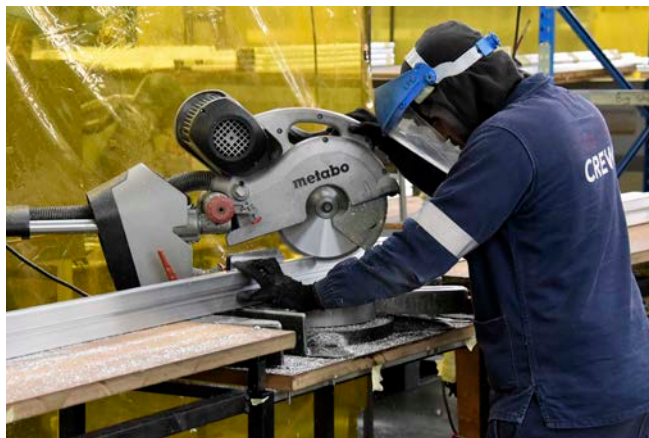
Alu-Cab does all its own in-house cutting to length of aluminium extrusions that are supplied by a local mill
