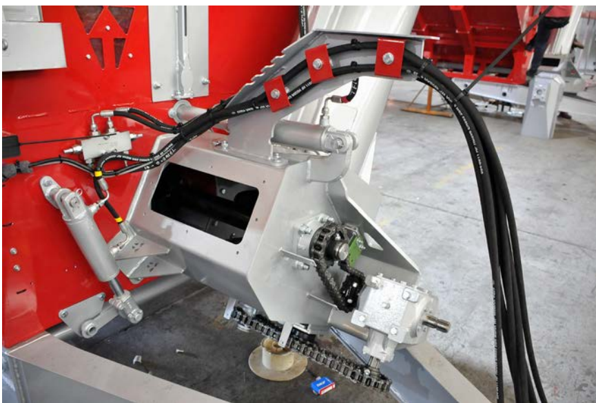
“The AgriCAD chaser bin’s hydraulically operated bottom dump gate enables rapid discharge into a silo receiving pit. The discharge auger has a capacity of around 5t/minute for rapid unloading to a height of 4.2m and the 3m wide bin makes unloading from the combine easier, minimising spillage.”
