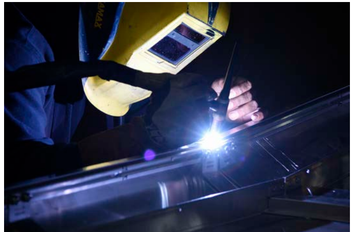
"We have stuck to MIG and TIG welding because it gives us the strength and aesthetics these welds provide that we are looking for with our products. Laser welding may look pretty, but if it's not structurally there, we are not going to take the risk of a customer who is driving down from Europe into Africa having a product fail in the middle of nowhere."
