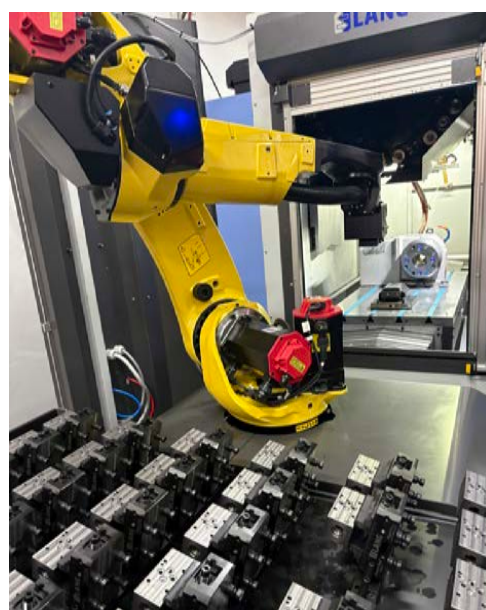
Miltek have 60 LANG Technik Makro•Grip® FS 77, 5-axis vises at their disposal, featuring jaw widths of 77mm, clamping ranges of 0mm – 120mm with continuous / full serration
