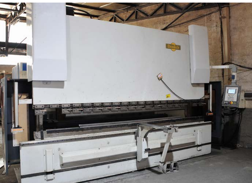
The company has a 150 ton press brake. Not being a high-volume service centre, they have adequate capabilities but will need to upgrade going forward. They process 90% of their sheet metal work in-house
