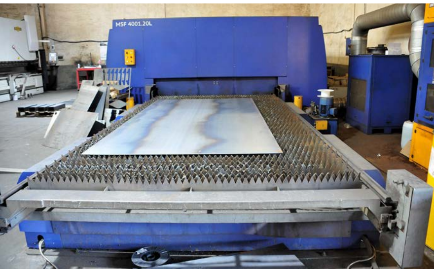
The company makes use of a fiber laser with a 4 by 2 metre bed
