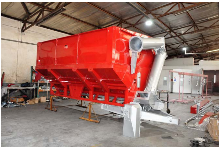
A chaser bin in the process of being fabricated
